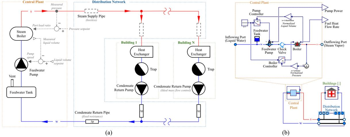
Figure 4: (a) Schematic diagram of the steam DH system with a central plant, distribution network, and  $N$  number of interconnected buildings and (b) Modelica diagrams of the complete DH system and central plant. The optional PRV in the building model is not included in this case study example.
