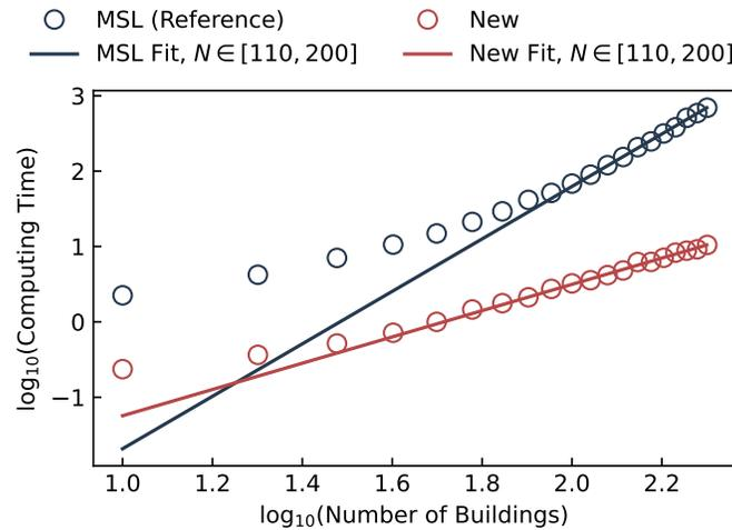
Figure 5: Computing time in seconds with respect to the number of buildings  $N$  and linear fits indicating scaling rates, on a log-log scale (base 10).
