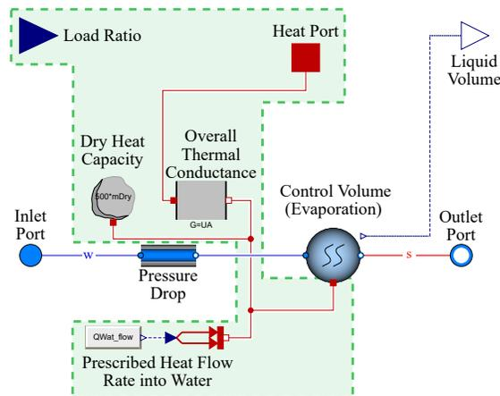
Figure 3: Modelica diagram for the steam boiler with an efficiency curve defined by a polynomial. Components in the green shaded region (including the heat port for the control volume, but not the volume itself) are conditionally removed if the boiler is configured with steady mass and energy balances.
