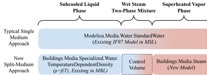
Figure 1: Water and steam modeling approaches. The liquid water model from the MBL calculates density  $\rho$  as a function of temperature  $T$ .
