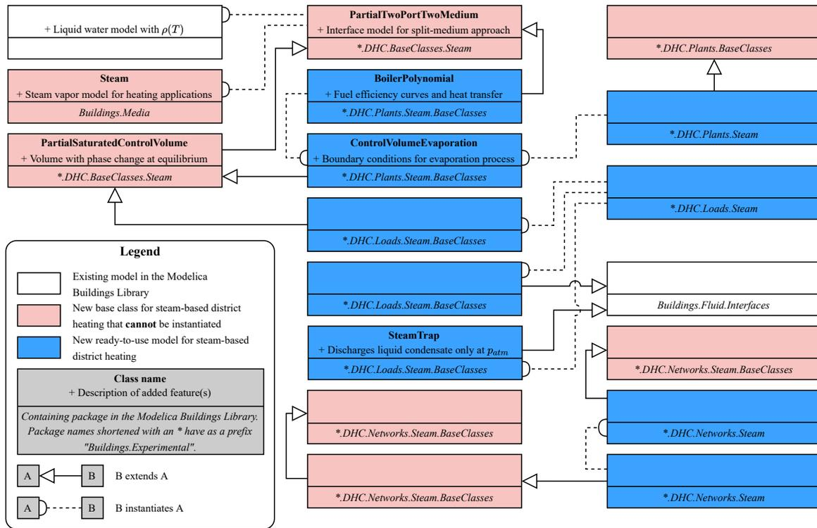
Figure 2: Class inheritance and instance diagram for the new steam district heating models in the MBL. Complete references to existing MBL models are not included due to space constraints. Note that the DHC package is located within the *Buildings.Experimental* package while it remains under development. This will later be moved to the *Buildings.Applications* package.
