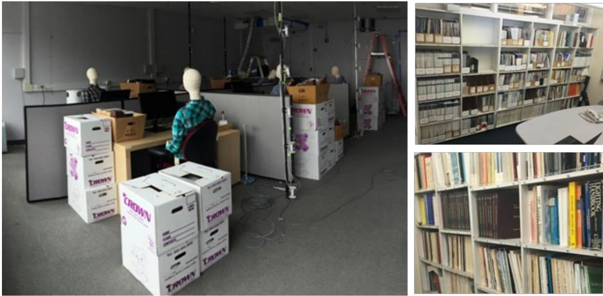
Figure 5 Experiment cell with about 1000 added books representing heavy internal thermal mass
