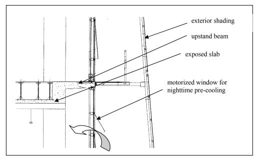
Figure 1. Section through slab/façade detail.
