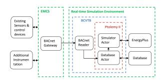
Figure 1 Overall system architecture
