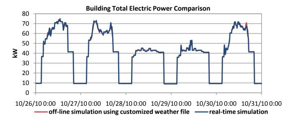
Figure 6 Building total electric power comparison between real-time simulation and off-line simulation using the customized weather file
