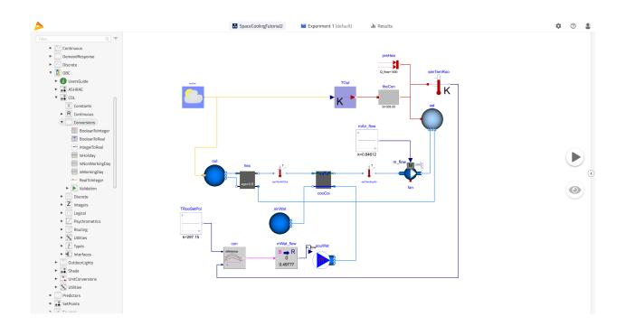
Finally, let's simulate the model for one day during summer from hour 4320 to 4344, and observe the response. First, edit the "Start Time" and "Stop Time" in the "Experiment" tab. Then, simulate the model and view the results.
