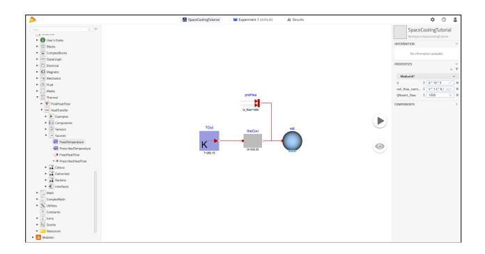
Finally, let's simulate the model for 3 hours, or 10800 seconds, and observe the response. First, edit the "Stop Time" in the "Experiment" tab. Then, simulate the model and view the results.
