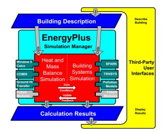
Figure 1. Overall EnergyPlus Structure
