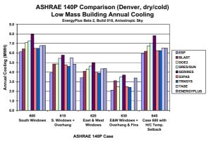
Figure 2. Sample EnergyPlus Comparative Testing Results
