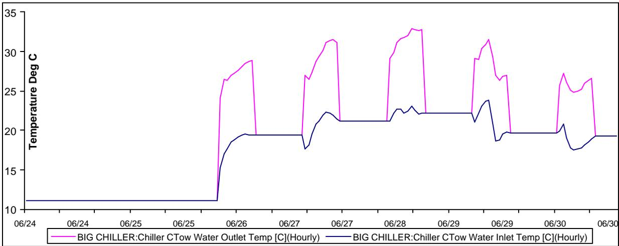
Figure 6: Cooling Tower Water Loop Temperatures
