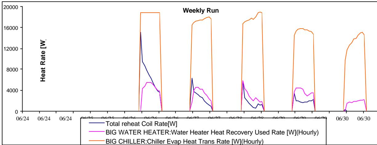
Figure 3: Evaporator Load on system
