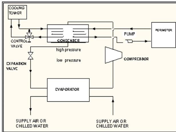
Figure 1: Diagram of General Electric Chiller with Heat Recovery.
