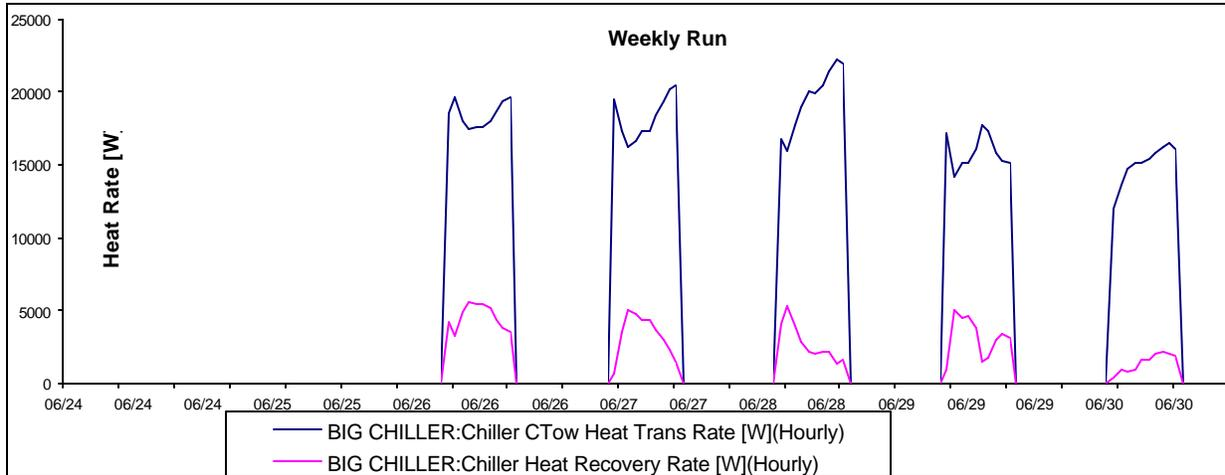
Figure 2: Cooling Tower Heat Transfer Rate and Heat Recovery Rate
