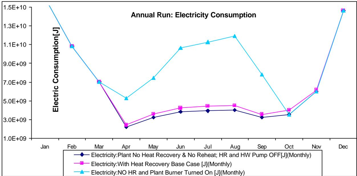
Figure 9: Heat Recovery & Non Recovery Cases
