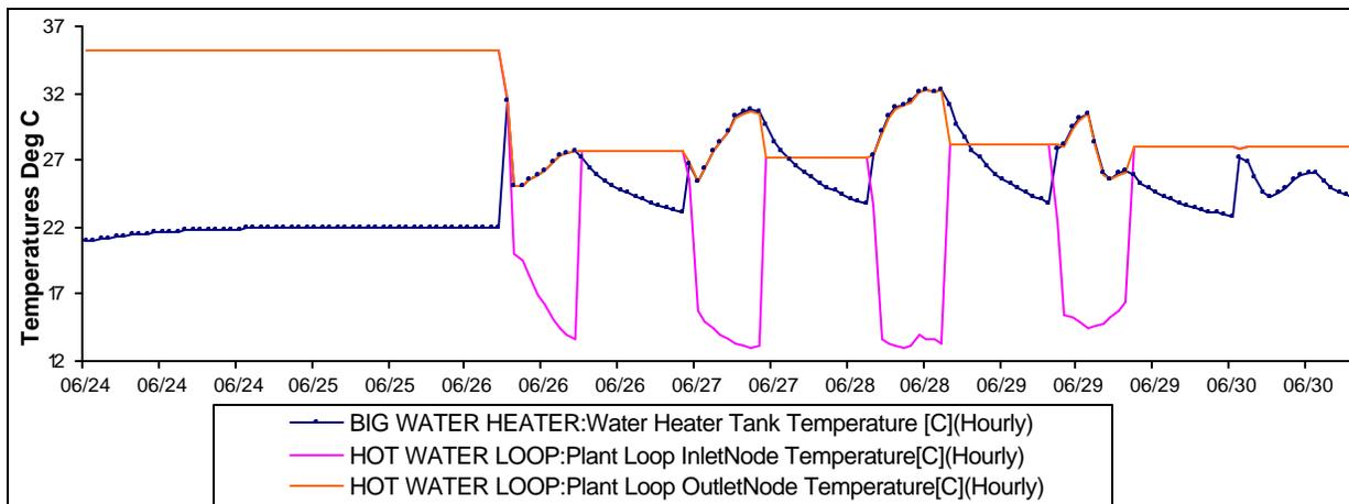
Figure 4; Temperature Variation of Hot Water Tank and Loops
