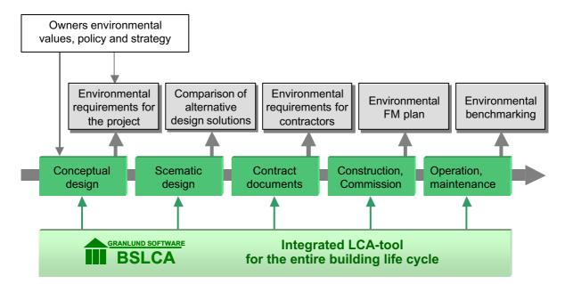
Figure 7. BSLCA is used through the entire building life cycle, from conceptual design to facilities management.
