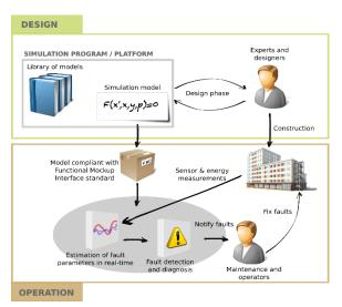
Figure 2. Model-based fault detection using state estimation techniques compliant with the FMI standard
