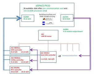
*Figure 3. Schematic of HiL setup.* generation.
