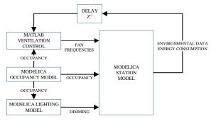
Figure 1. The Modelica Model-in-the-loop simulator
