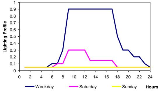
Figure 2. Lighting schedule with occupant sensor control
