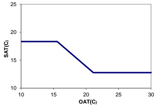
Figure 5. Stepwise function for supply air temperature reset based on outdoor air temperature
