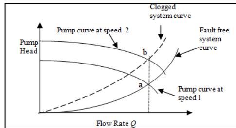
Figure 1 Effect on clogging on loop system curve
