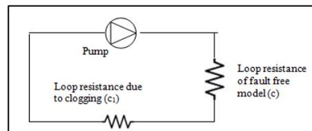
Figure 2 Plant loop resistances
