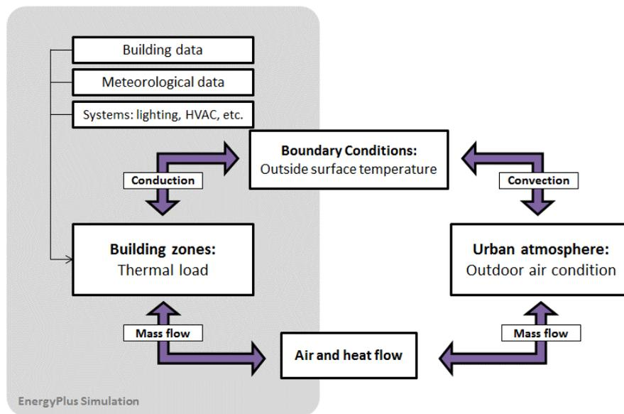
Figure 4. EnergyPlus data exchange with the urban atmosphere model
