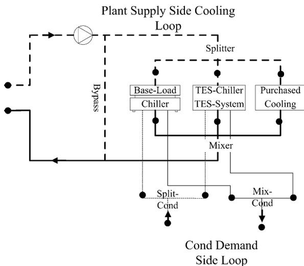
Fig. 1. Integration of base-load chiller, TES chiller, and TES system models within EnergyPlus Plant Supply Side Cooling Loop.
