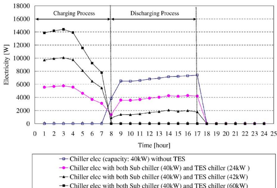
Fig. 6. Chiller electricity use for with/without TES plant on 21 July in Phoenix, Arizona.
