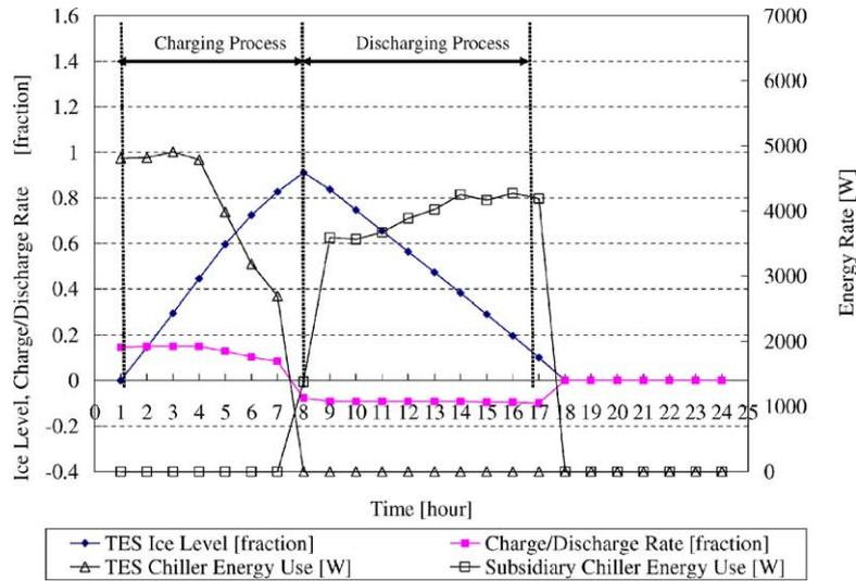
Fig. 5. Performance of the TES system using storage-priority: charge/discharge rate, ice level, and chiller energy use.
