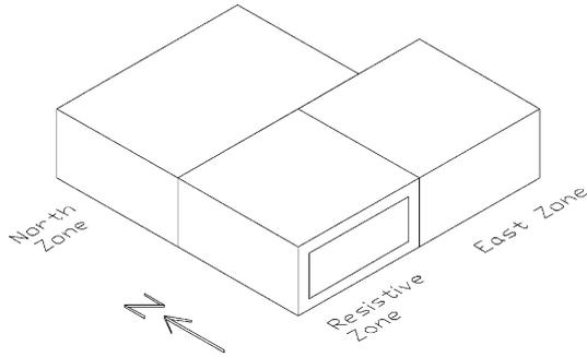
Fig. 3. Illustration of three-zone building model.
