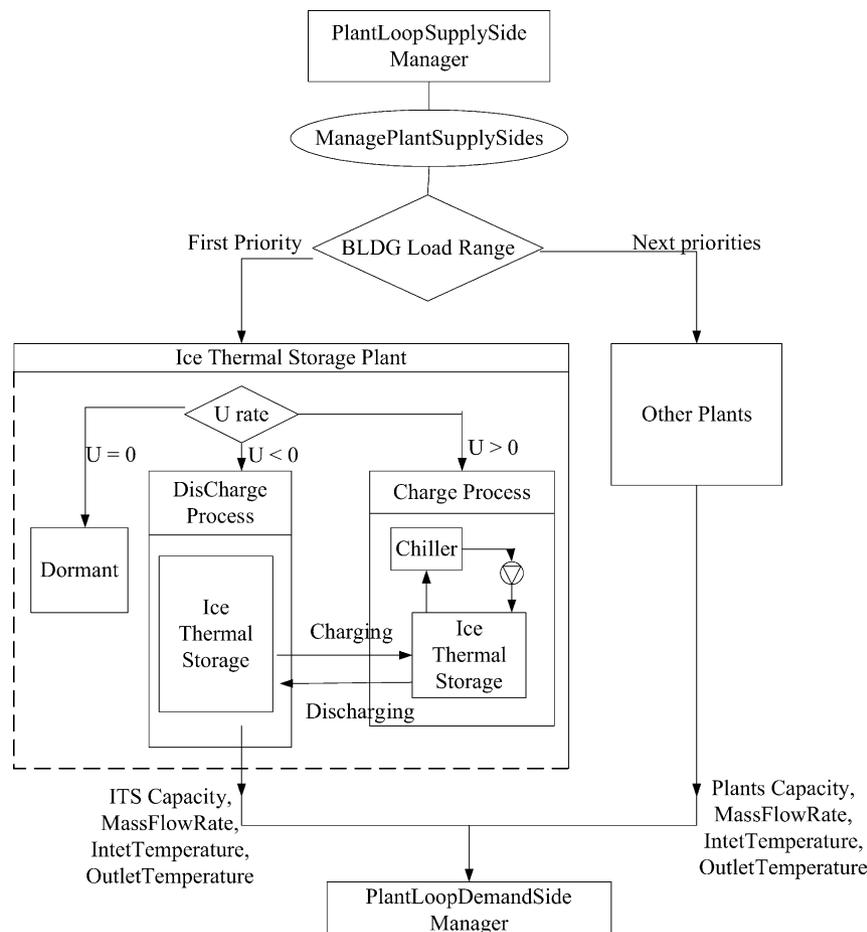
Fig. 2. Flow chart of operating processes and implementation of ice thermal storage plant model in EnergyPlus.
