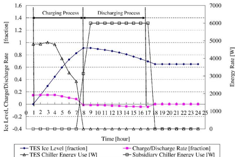
Fig. 4. Performance of the TES system using chiller-priority control: charge/discharge rate, ice level, and chiller energy use.
